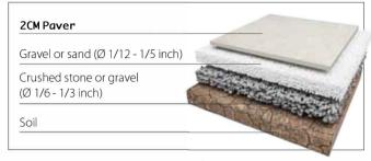
Recommended for larger areas, for installation with thin joints or joints without grass.
