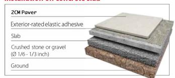
Installation with thin set on concrete slab recommended for areas open to vehicular traffic or subject to very high stress: leave joints at least 1/8 inch wide and respect expansion joints.
