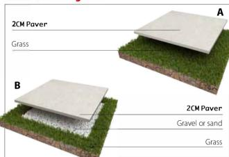
Installation on grass can be performed in two ways:
