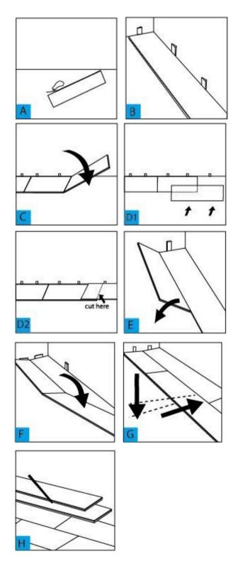
Remove the tongue (on the long side) from the first row of planks. This will ensure that the decorative surface of the flooring is under the finished trim when installed. Use a utility knife to score through the tongue several times until it easily snaps off (Figure A).
